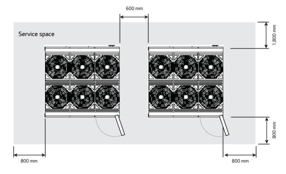
2020 LG HVAC Solution | 35 34 | 2020 Air Cooled Inverter Scroll Chiller
